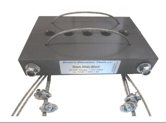
All car or counterweight hitch plates have a staggered hole pattern that allow sufficient space to fit and adjust the rope shackles. The ropes lead off from the car or counterweight hitch plate with as much as a 4-inch spread with each rope running in its own straight line to where it makes contact with the sheave.
